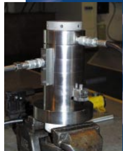
Test charging a custom-built HydraJAC.
