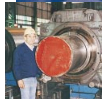
The S12402 HydraSure Clamp Nut is one of the larger sizes developed for use in the Port Kembla works of BHP Steel. Specifically engineered for this duty, it is applied to the roll shafts of the plate mill at the steelworks. It is shown here installed on a roll stand.
