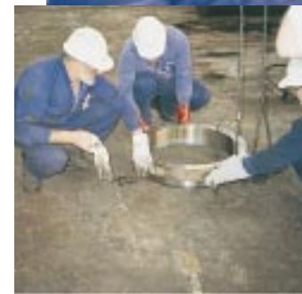
HydraSure Clamp Nut used in steel rolling mill.
