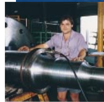
HydraSure Clamp Nut during test fitting to shredder shaft for sugar mill.
